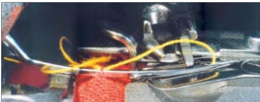
Needle in loop pick-up position. The fibres which were separated from the fabric by the fine needle point, wrap around the needle blade.
