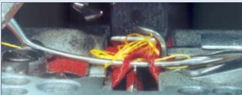
The ball point found its path right through the fabric in a complete penetration. The consequence is a "throughstitch" instead of the intended blindstitch.
