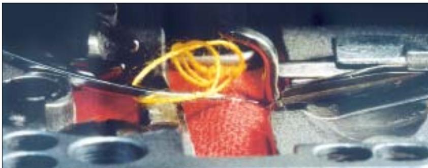
Needle point has entered fabric. Split-off fibres are shifted up on the point cone.
