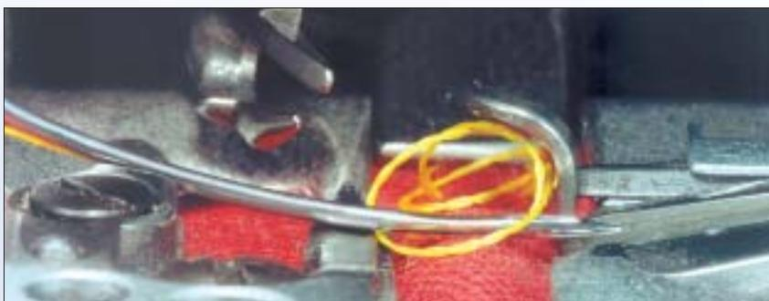
Needle just before penetration. The ball point has impeded the separation of fibres from the cloth as it caused the needle to deflect. A skipped stitch is the consequence .
