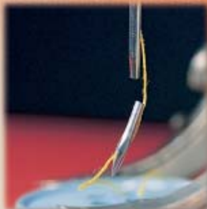
2 The needle can bend and break.
