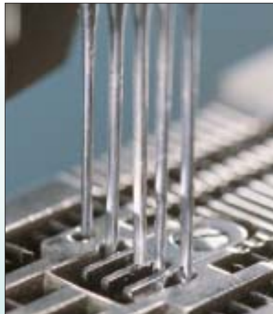
A broken needle crashes upon a stitch finger
