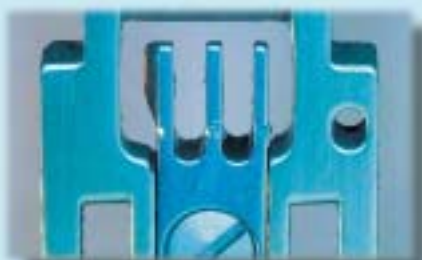
Damaged throat plates
