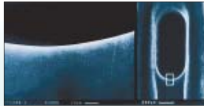
The string polished eye surface of a Groz-Beckert needle
