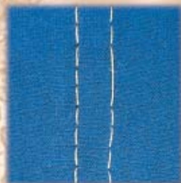
Skipped stitches, staggered seams
