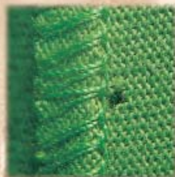
Fabric damage (needle cuts)
